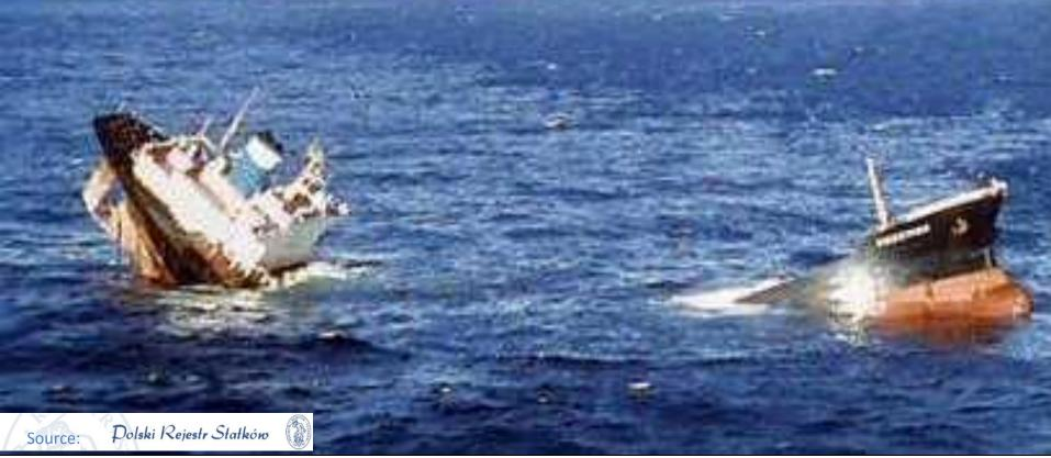
In 1999, the tanker "Erica" broke up on passing the French coast causing an environmental disaster. The causes underlying the incident lay in the bad technical condition of the hull structure.
